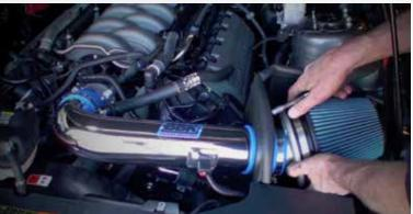
Remove the air inlet tube and set it aside.
