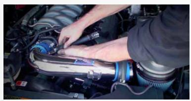
Disconnect the smaller plastic breather tube from the air inlet tube. You can leave the sound tube connected.
