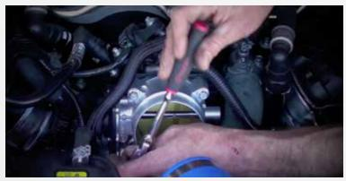
Remove the four mounting bolts from the stock throttle body, as you remove the throttle body, flip it to unplug the motor plug on the bottom.
