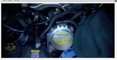
Re-install the air inlet tube and reconnect the breather tube. A little WD-40 or light grease on the inside of the tube may help in this process. Tighten the clamps.
