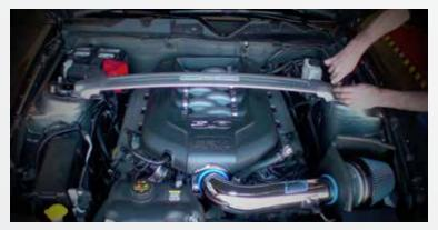
Remove the strut tower brace if applicable.
